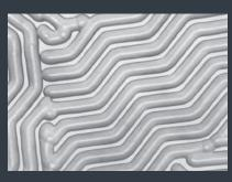
Micro-engraving Line width 20µm, depth 10µm Courtesy of Karmic Sàrl
